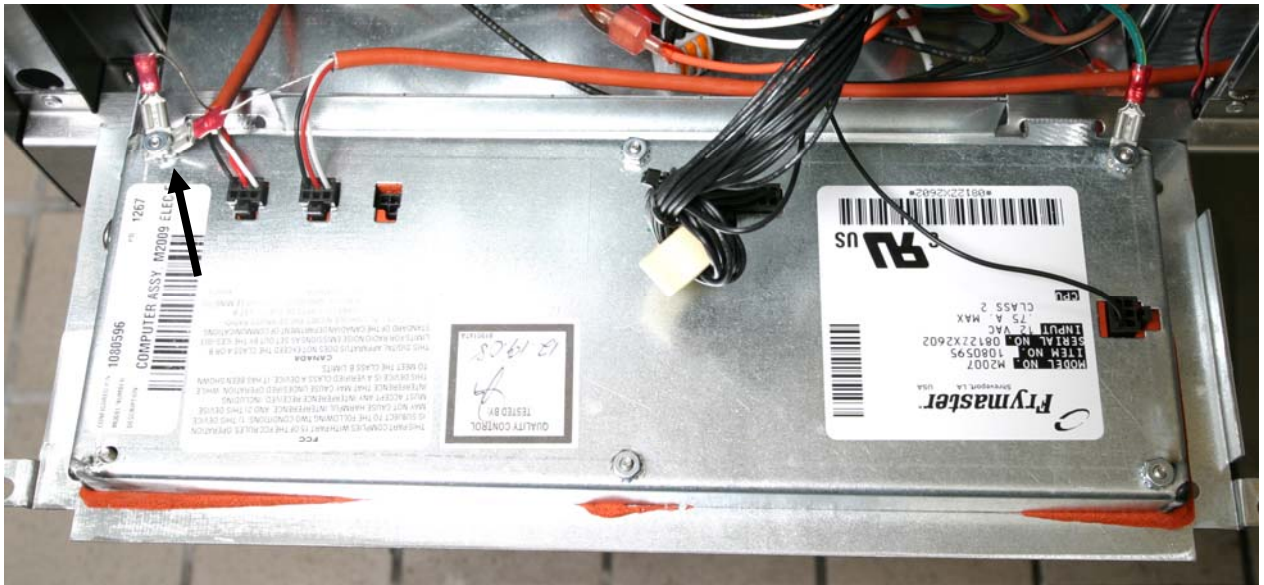
Figure 7: The computer is shown with its grounds reconnected. The data-cable grounds on the left must be in place.
